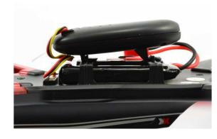
6. Plug the camera in to the WiFi port on the bottom of the Quadcopter. The WiFi port is the only connector with 3 connections.
